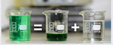
Evaporation allows for an extreme concentration of effluents and the production of condensates, which can be recycled or discharged into the natural environment.
